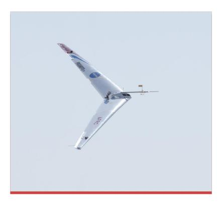
That's the "Prandtl-M", a reference model, designed to fly in low pressure conditions (7-9 hPa on Mars)
