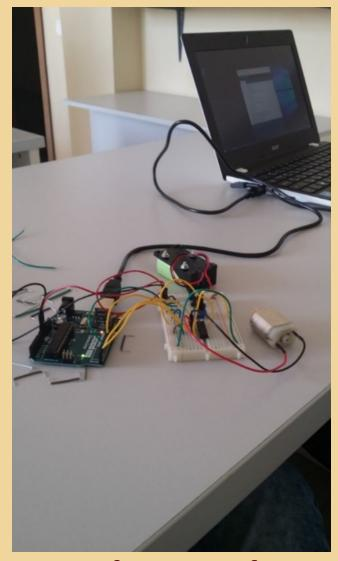
The Arduino boards, by which alone the system of motors of LEGO – models of the Mars Rovers
